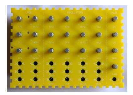
Time to test The Bumblebee! Plug it with a power chord (+@ring, -@tip for the 2.1mm connector) and check that all its elements are working .
