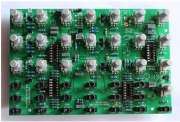
Now solder the power connector. If you want to use The Bumblebee with the desktop case solder the 2,1mm. If you want to use it on an eurorack system solder one of the 2 other connectors. Insert the ICs. Check polarity!
