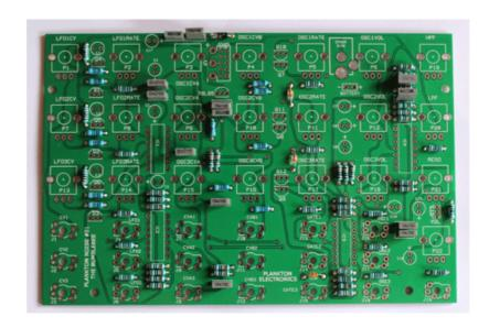
Solder the electrolytic caps. These are the cilindric ones. But we will solder these ones to the rear part. Take in mind that these capacitors are polarized, so you must respect the orientation. The long led corresponds to the positive "+" side. The negative "-" side is also marked with a visible white line.
