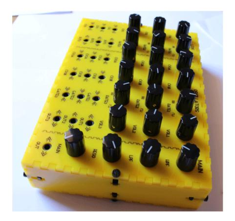
As you can see, before insert the top panel you have to screw the PCB to it via the potentiemeters with its nuts. You can mount the knobs when the case is ready.
