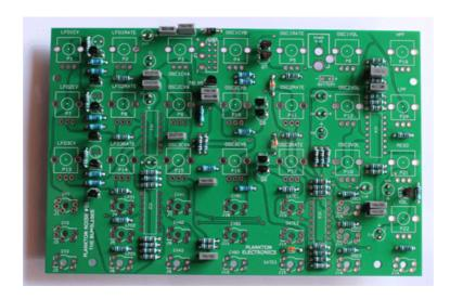
Now solder the IC sockets. The mark on one of the sides points to the first and last pin. This one should face up.
