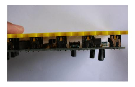
Time for the potentiometers now. First of all we need to take the nut and the washer off. Then we have to remove the small tab in the top part of the potentiometer. Use a small pliers to do it.
