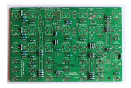
We will follow soldering the film capacitors (the rectangular ones). Start with the 10n (103) and continue [82n (823), 100n (104), 220n (224) & 330n (334)]. Then we will solder the 4 diodes. Note that the diodes have an orientation marked with a stripe that's also on the PCB.
